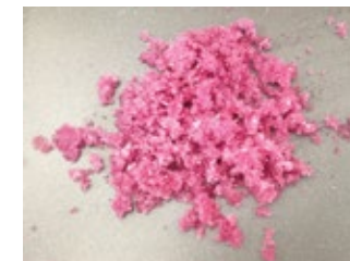
4) Spilled liquid has been neutralized & absorbed
