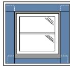
Apply the final top horizontal piece of BT25XL on the top of the window fin.
