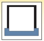
Apply Protecto Sill Pan Flash into the rough window sill prior to setting the window.
