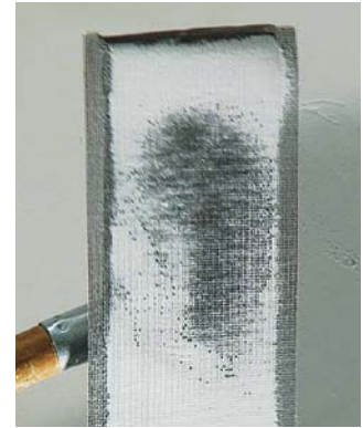
Other low-dust products can clog, polishing the finish and leading to paint flashing.
