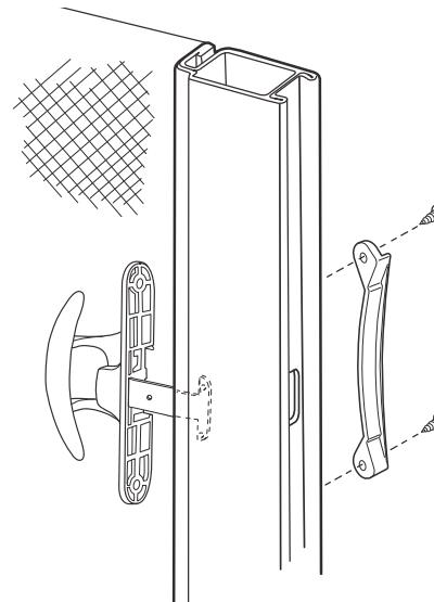
Remove old handle. Slide inside handle (1) into frame feeding hook through slots in frame. Install outer handle in old location (2). Install screws.
