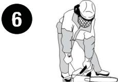
Place right foot in rear handle as shown. Using right hand, pull starter rope sharply until machine starts, or a maximum of 5 times.
