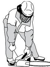
1. Lay the chainsaw on a flat surface. The cutting attachment must not be in contact with the ground.
