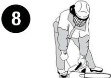
Pull starter rope until engine starts.
