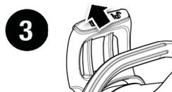
Make sure chain brake is locked by pushing forward on handguard.
