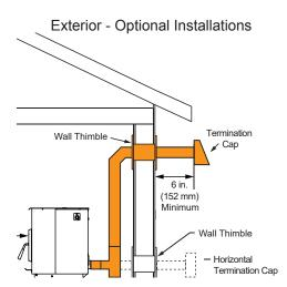
NOTE: In Canada when using a factory-built chimney it must be safety listed, Type UL103 HT (2100<sup>0</sup>F) CLASS "A" or conforming to CAN/ULC-S629M, STANDARD FOR 650°C FACTORY-BUILT CHIMNEYS.
