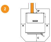
Non-combustible floor protection extending beneath the flue pipe is required with horizontal venting or under the top vent adapter with vertical installation.
