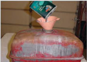
Step 3: After the tank is clean, drain the tank and rinse thoroughly with water. Let the tank dry. When totally dry, pour in the can of Fuel Tank Sealer .
