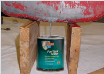
Step 4: After all surfaces have been coated, drain the tank for about an hour to remove excess sealer from the tank.
