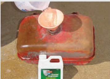
Step 1: Mix 1 quart Cleaner Degreaser with one quart of hot water. Use this solution to remove any gum, varnish or sludge from the inside of the tank.
