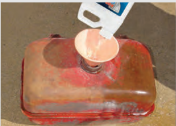
Step 2: Pour in the entire bottle of Metal Prep to dissolve rust, coat the tank with zinc phosphate, and etch the metal for better adhesion of the sealer.
