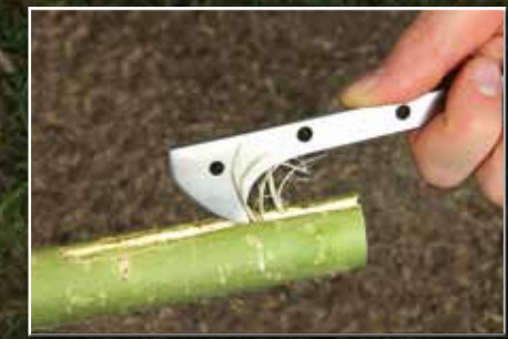
Hawkbill-shaped inletting tool is used to carve a slot for tying the Harpoon onto any green shaft.
