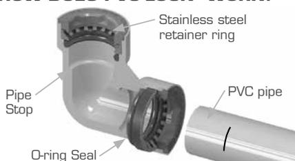
When PVC pipe is inserted to the Pipe Stop, the o-ring seals around the pipe and the stainless steel ring “locks” the pipe in place.
