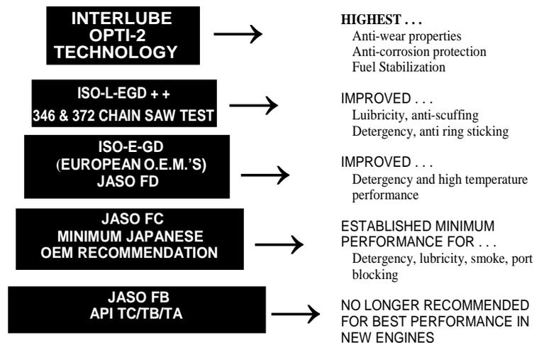
THE DEMANDS ON TWO CYCLE ENGINES HAVE INCREASED DRAMATICALLY RESULTING IN A PYRAMID OF LUBRICANT PERFORMANCE LEVELS.
