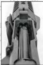
Insert scraper into star chamber and twist to scrape
