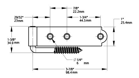
Blind Hinge Pack consists of four screw pintles, four hinge straps Material: Steel Finish: Black Finish Fasteners: (12) Wood Screw, Flat Head, #8 X 1.0"
