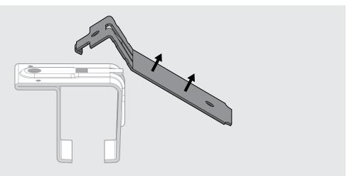
If the flashing bracket will be installed again on a rail bracket, you may need to use a flathead screwdriver to bend the locking tab back to its original position.
