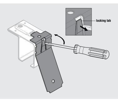
Remove the flashing bracket.
