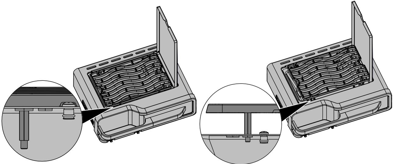
**Cooking Grid Placement:** The cooking grid can be placed at two different heights. The lower height is for use with pots or pans. The higher position is to be used when searing meats. Ensure the burner is off and the grid is cool to the touch before changing between the two heights. The grid must be at the lower height in order to close the lid.
