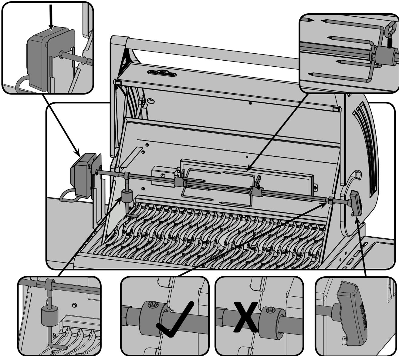
Ensure stop bushing is tightened on the inside of hood casting.
