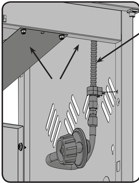
Ensure the regulator drops into the small opening, between the tank heat shield and the right side of the cabinet.
