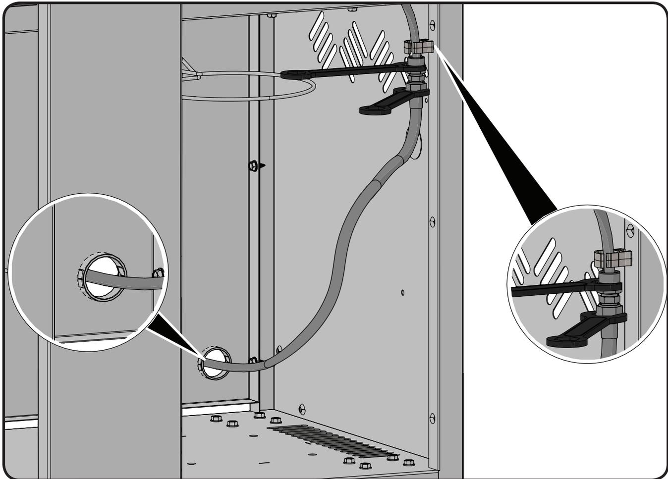
**Clip hose to side panel using hose retainer clip supplied.**
