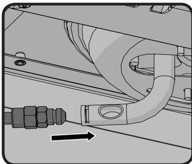
Fit orifice into burner tube and secure with hose retainer clip supplied.
