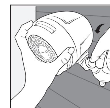
4. Loosen the knuckle screw located on the stem of the light to point the light in desired direction. Then tighten the screw to secure position.
