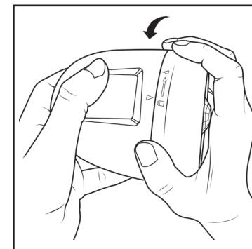
1. Remove the front cover of the spotlight by rotating the face counterclockwise. Pull the face out from the housing to reveal battery holder.
