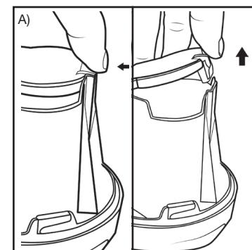
2. A) To release the door on the battery compartment, use your thumb to press the tab into the light and lift the door off the light.
