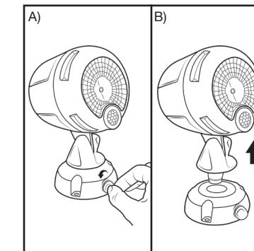
1. A) Remove the mounting base by turning the thumbscrew counterclockwise.
