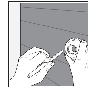
2. Determine the mounting location and mark the pilot holes. Use a 1/16" drill bit to create the pilot holes (if mounting to drywall, use the plastic anchors included with the screws). Use a hammer to tap the plastic anchors into the pilot holes before screwing in the mounting base.
