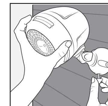
3. Drill the screws through the holes on mounting base. Insert the stem back into mounting base and tighten the thumbscrew.
