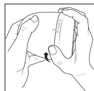
3. Line up arrows then turn the face of the light clockwise. Make sure the unit is closed by twisting until the arrow symbol is pointing past the lock symbol, to ensure weatherproof seal is tight.
