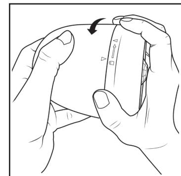
1. Remove the front cover of the spotlight by rotating the face counterclockwise. Pull the face out from the housing to reveal battery holder.
