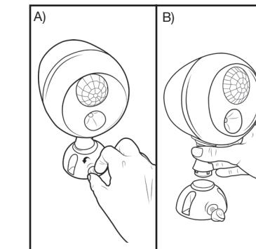
1. A) Remove the mounting base by turning the thumbscrew counterclockwise.
