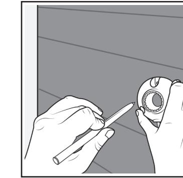
2. Determine the mounting location and mark the pilot holes. Use a 1/16" drill bit to create the pilot holes (if mounting to drywall, use the plastic anchors included with the screws). Use a hammer to tap the plastic anchors into the pilot holes before screwing in the mounting base.
