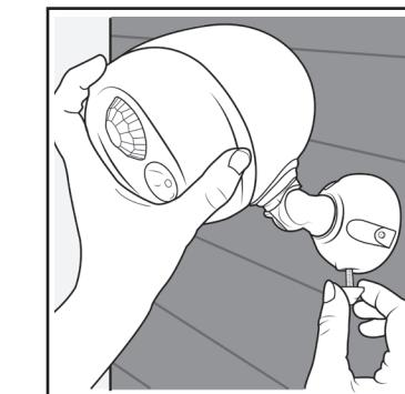
3. Drill the screws through the holes on mounting base. Insert the stem back into mounting base and tighten the thumbscrew.
