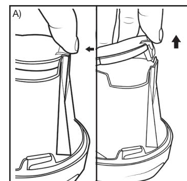
2. A) To release the door on the battery compartment, use your thumb to press the tab into the light and lift the door off the light.
