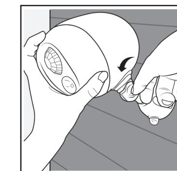
4. Loosen the knuckle screw located on the stem of the light to point the light in desired direction. Then tighten the screw to secure position.
