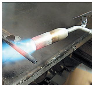
The HT torch is great for heating flat iron or metal tubing.
