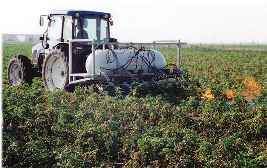
The patented liquid spray flaming process in action.
