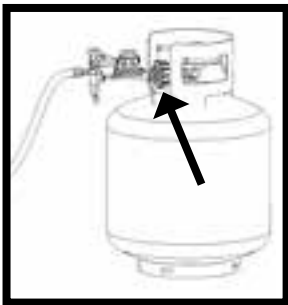
Apply solution to gas cylinder valve.
