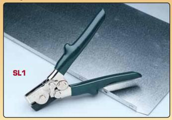
Join sheet metal, duct and pipe sections economically. No need for extra hardware. Punches raise a louvered shaped projection on metal edge for locking into rolled edge of sheet or piece to be joined. Metal pieces snap together and are fastened securely. Compound Handle
