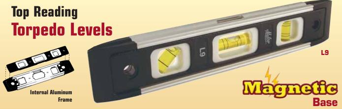
Duplex milled aluminum frame with "cycolac" end plates is lightweight and withstands shock or abuse. Precision cast parallel edges will not scratch work surface. Three large vials - plumb, level and 45°. White vial holders and top read feature facilitate quick, easy reading. Grooved working edge designed for use on pipe and conduit.
