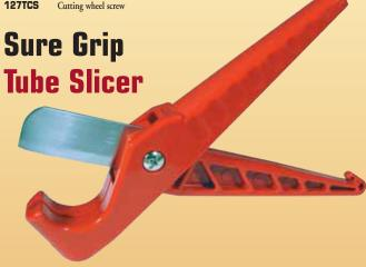
Produces cuts in ABS, PVC, rubber and fabric reinforced hose up to 1" (25.4 mm) I.D. Rigid, durable nylon handle design provides sufficient leverage when cutting so that only moderate hand pressure is required. Stainless steel cutting blade is resharpenable and replaceable.
