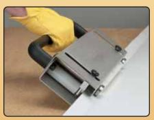
Slide tool over edge of metal and make a score by gliding tool along full length of panel.
