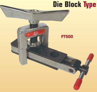
For soft copper, aluminum and brass tubing. Faceted, hard chrome finished cone rolls out perfect 45° flares - then automatically burnishes flare face. Handy slip-on yoke permits use in tight quarters. Movable dies allow tubing to be slipped in easily. Heat treated dies grip tubing without scoring and the original tube wall thickness is maintained at base of flare. Satin chrome and black nickel finish.
