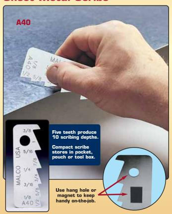
Scribe commonplace trim lines on galvanized sheet metal quickly and accurately. Ten pre-set scribing depths from 1/8" to 1"(3 to 25 mm). Each scribing depth size features a dual edged point to create clean, readable and accurate score lines parallel to the edge of the metal sheet. Corrosion resistant finish and etched-in dimensions are readable for life of tool. Packaged in a clear vinyl, reusable pouch for storage in pocket, pouch or tool box.
