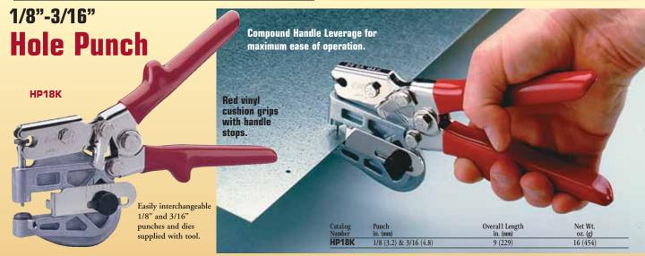
Does the work of more expensive bulkier punches faster and easier. Work overhead to pre-punch rivet holes in suspended ceiling grids or use in any edge application for making holes in window extrusions, metal ductwork or sheet stock. Compound leverage increases one hand mechanical advantage 8 to 1. Spring return handles allow quick set-up for repetitive applications. Stop gauge permits adjustments from 1/4" to 1-1/8"
