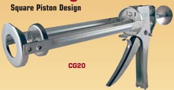
Heavy duty professional models with thumb-activated pressure release. Designed for use with spouted cartridge. Powerful ratcheting action minimizes worker fatigue or need to warm up caulk. User can regulate stroke to fit hand. Square piston rod may be rotated to expose new gripping surface and increase service life of tool. Handy puncture wire folds inside handle.
