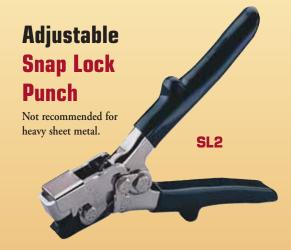
Slide adjustment for throat depth allows settings from 1/4" to 5/8" (6.35 to 15.88 mm) depth. Also used to crimp end caps on gutter. Nickel plate and black oxide finish. Green grips. Formed metal cutting jaws.
