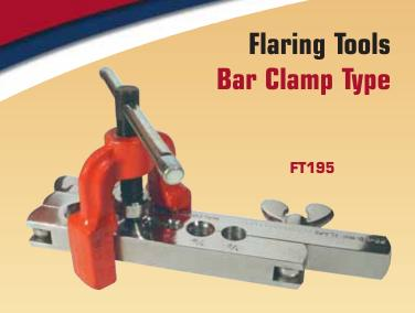
Flares 7 sizes of soft copper, aluminum and brass tubing. Forged steel slip-on yoke and hardened flaring bar. Yoke design permits flaring where there is little space between nut and tube end. Positive clamping of bars prevents tube slippage. Hard chrome-finished swivel-type cone makes better flares with less effort. Satin finish nickel-chrome plated.
