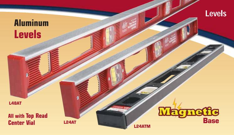
Strong and durable extruded aluminum frame is heat treated and grooved on both gauging surfaces. Unique construction design features multi-directional vial. Dust proof covers are screwed in to protect vial. Top read feature makes for quick, easy reading. Available in 24" (61 cm) and 48" (122 cm) lengths.
