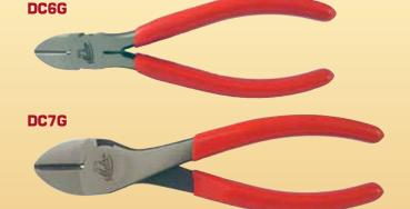
Powerful leverage short nose is designed to cut flush from side without obstructing handle grip. Absence of flat gripping surface on jaws allows tool to cut out to very tip. (Diagonal cutters are the only tools capable of reaching into an electrical box to cut wires). Smooth functioning box joint insures accurate alignment of cutting edges. Forged from high quality alloy steel. Hardened and tempered for long life. Polished faces. Red vinyl cushion grips.
