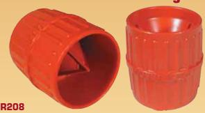
For copper, aluminum and brass tubing. Reams both inside and outside edges of tube with 3 hollow ground tool steel blades. Tool cuts when turned both clockwise and counter-clock-wise. Fluted body is shaped to fit comfortably in palm.
