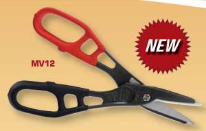
Lightweight 12-inch (31 cm) Combination Snip, with BIG 3-inch (76 mm) cutting depth. A knife-like edge produces a smooth slicing action for cutting thick or layered vinyl and a variety of other flexible non-ferrous materials.
