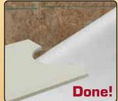
Notcher may then be used to cut all the way through plank along pre-scored line.
