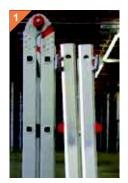
Release the lock assemblies, and pull the inner ladder assembly completely out of the outer ladder bases.
