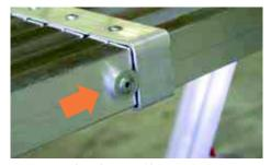
This safety feature (Stopper) on the telescoping plank keeps the plank sections from separating.
