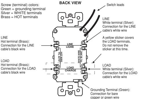
(a) Detach two of the cable's white and hot wires from the receptacle and cap each one separately with a wire connector. Make sure that they are from the same cable.
