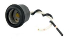
Incandescent lampholder, medium base, single circuit, 660W-250V; black rubber; with shoulder for clamp type shade; with two 6 inch 16AWG black and white leads, free ends stripped 3/4 inch.
