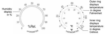
The thermometer and hygrometer have been calibrated at the factory. To check the sensors accuracy, tune to your local weather forecast information broadcast for the latest weather information. The sensors may be adjusted.
