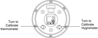
To manually adjust the sensors, gently turn the temperature or humidity sensor adjustment at the back of the clock until desired setting has been reached.
