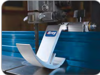
Add a stop to the fence for repeat cuts to a set depth, such as cutting tenons.
