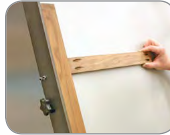
Flush Face Frames Made Easy: 1) Align stile and rail along squaring fence 2) Adjust clamp cylinder and secure joint line 3) Drive self-tapping screw
