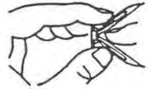
Fig. 18 - Popping Open Anchor Wing For Thin Walls
