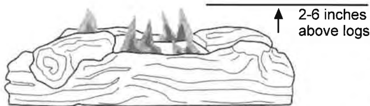
Fig. 31 - Correct/Normal Flame Pattern with short flames
