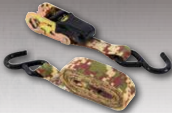
83102 12' x 1" Ratchet Tie-Down, Digital Desert Camo 500 lbs. WLL 1,500 lbs. Break Strength
