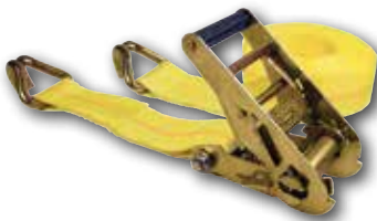
04629 25' x 2" Ratchet Tie-Down, 4 pack 3,333 lbs. WLL 10,000 lbs. Break Strength
