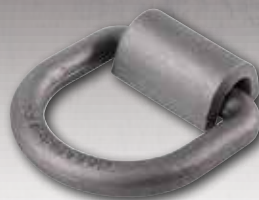
89318 5/8" Surface Mount Weld-On D-Ring Anchor 5,000 lbs. WLL 15,000 lbs. Break Strength Package: Bulk/Cut Case Ship Pack 8
