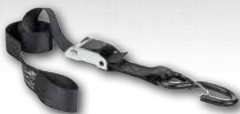
07501 Bow Safety Strap, 1.25"x4' 400 lbs. WLL 1,200 lbs. Break Strength
