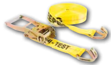
04630 30' x 2" Ratchet Tie-Down 3,333 lbs. WLL 10,000 lbs. Break Strength
