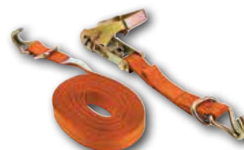
05516/89516 16' x 1" Ratchet Tie-Down 1,000 lbs. WLL 3,000 lbs. Break Strength
