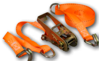
05515/ 89515 15' x 1" Ratchet Tie-Down 666 lbs. WLL 2,000 lbs. Break Strength
