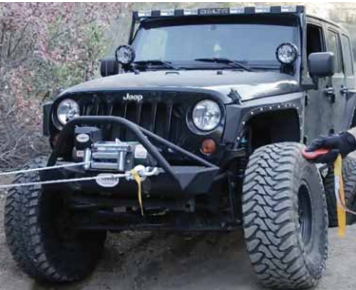
KW17.5 12VDC 17,500 lb Winch
