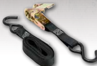
05511/ 89511 10' x 1" Ratchet Tie-Down 300 lbs. WLL 900 lbs. Break Strength
