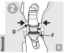
On socket that is to be replaced, press sides of socket shell (D); rock shell back and forth and lift up to remove from socket cap (F).
