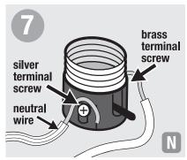
Connect ribbed neutral wire (feel outside of cord for ribbing) around silver terminal screw. If no ribbing, determine neutral wire and connect around silver terminal screw. Connect smooth wire around brass terminal screw.
