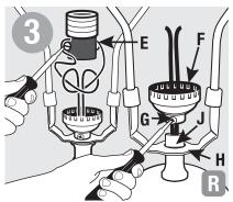
Unscrew terminal screws (E) to release wires. Unscrew socket screw (G). Unscrew old cap (F) from lamp nipple (J) and remove.
