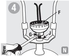
Insert wires through bottom of new socket cap (F). Thread new socket cap onto lamp nipple (J) and tighten. Tighten socket screw (G). Cardboard insulation disc should be firmly in bottom of socket cap (F).
