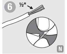
Using wire stripper, expose 1/2" of bare copper strands from cord. Twist copper strands tightly together.
