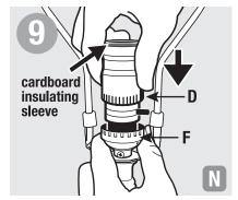
Ensure cardboard lining is in place, then fit socket shell (D) into socket cap (F) by gently rocking side-to-side, until shell snaps into place with clicking sound.
