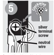
Connect the white or ribbed wire around silver terminal screw and other wire around brass terminal screw. Wrap each wire clockwise 34 turn under head of screw and tighten screws. Cut loose strands.
