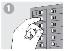
Before beginning TURN OFF POWER to the light from fuse or circuit breaker.
