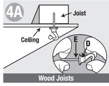
Thread hanger bolt (E) into swag hook (D). Tighten until hanger bolt reaches bottom of hole in swag hook. Screw entire ensemble into joist until flush with ceiling.
