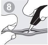
Cleanly cut non-ribbed wire in half at center of slit. Do not strip wire.
