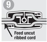
Place uncut ribbed cord in open channel of hollow half of switch. Tuck two cut ends of non-ribbed cord into top portion.
