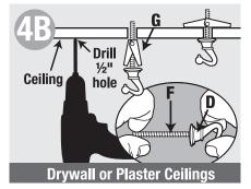
Drill 1/2" hole into ceiling. Thread threaded stud (F) into swag hook (D). Tighten until threaded stud reaches bottom of hole in swag hook. Thread threaded stud through channel side of spring toggle wing (G). Fold wings downward and push through drilled hole. Tighten until swag hook is securely in place and flush with ceiling.
