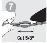
Where switch is to be located, cut 5/8" slit through insulation between conductors. Do not expose wire.
