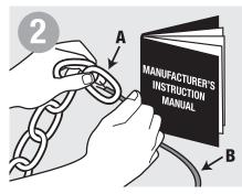
Thread the spliced end of cord (B) through chain (A) by going through every 4th or 5th link. Connect cord to fixture, following recommended fixture manufacturer's instructions.
