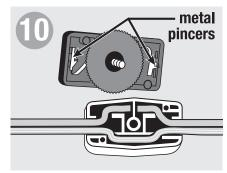
When switch halves are combined, cut portion of wire should contact metal pincers.
