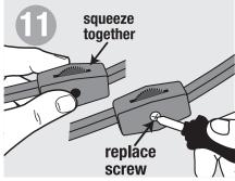
Place two switch halves together until they touch. Replace screw; securly tighten nut.
