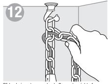
Slide chain onto swag hook. Support weight of luminaire or fixture by the chain, not wire. Do not drape wire over hook.
