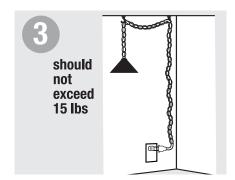
Determine placement of light. It is best to screw into stud, but toggle bolt can be used on plaster or drywall ceiling that is structurally sound to support minimum of 30 lbs. Weight of all materials should not exceed 15 lbs.
