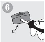
Unscrew nut to separate switch (C).
