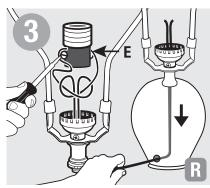
Unscrew terminal screws (E) to release wires. Pull old cord through bottom or side of fixture to remove.
