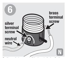
On the socket, connect ribbed neutral wire (feel outside of cord for ribbing) around silver terminal screw and smooth wire around brass terminal screw.
