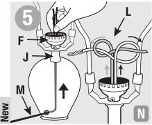
Feed cord (M) through bottom or side of lamp, up through nipple (J) and out socket cap (F). Cardboard insulation disc should be firmly in bottom of socket cap. Tie an Underwriter's knot (L).
