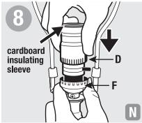
Make sure cardboard lining is firmly in place in socket shell (D). Place socket shell on cap (F). Pull extra wire back through lamp. Snap socket shell into socket cap by gently rocking side to side, until shell snaps into place with clicking sound.
