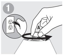
Before beginning **TURN OFF POWER** by unplugging lamp from wall outlet. Unscrew finial (A), remove lamp shade and bulb.
