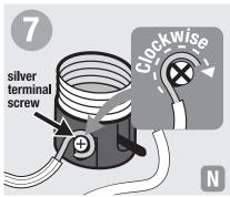
Wrap each wire clockwise 3/4 turn under head of terminal screw and tighten screws. Cut loose strands.
