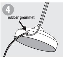
If feeding through metal lamp base, make sure rubber grommet is in place. Replace if needed.
