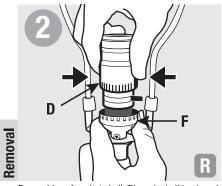
Press sides of socket shell (D); rock shell back and forth and lift up to remove from socket cap (F).
