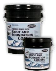
A fiberized asphalt emulsion designed for coating a variety of roof surfaces and concrete foundations. Dries black.
