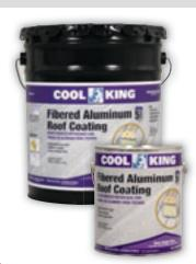
A blend of pure waterproofing asphalt and high grade aluminum pigments plus the addition of fibers. Reflects up to 80% of the sun's rays, helping prevent excessive drying and cracking of substrate, thus reducing leaks. Areas immediately under roof will remain approximately 15-20 degrees cooler in summer. In winter, inside heat is reflected back into the building, thus saving energy costs. Dries silver.
