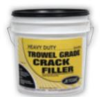
Heavy-bodied sand-filled trowel grade asphalt emulsion crack filler designed for filling cracks up to 1" wide in asphalt pavement surfaces. Can also be used to fill shallow ruts and depressions in pavement surfaces.
