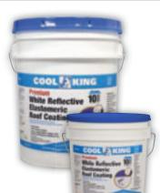
A 100% acrylic, highly elastomeric, titanium fortified roof coating formulated to provide a high solids rubber-like membrane. Designed for use on metal, polyurethane foam, EPDM, APP, masonry, asphalt and wood surfaces. Forms a highly reflective barrier resulting in significant energy savings. Dries bright white.
