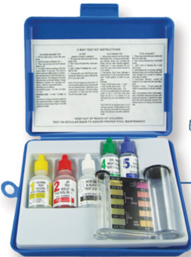
00-486 Deluxe Test Kit 4-Way, 5-Factor, OTO Test Kit, Cl, Br, pH, Acid Demand, Alkalinity
