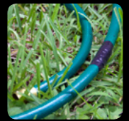
Wrap hoses for an airtight seal
