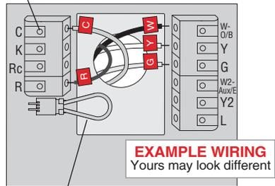
Remove jumper loop **ONLY** if you have both **R** and **Rc** wires.
