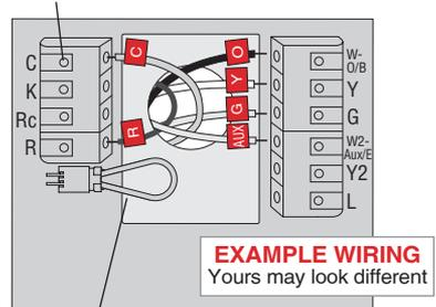
Remove jumper loop **ONLY** if you have both **R** and **Rc** wires.
