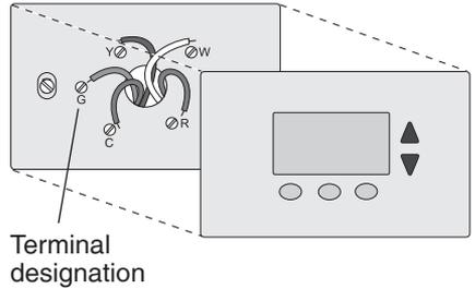
**Important!** C wire is required and is the power source for your thermostat. Without a C wire, your thermostat will not power up.
