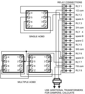
TRANSFORMER SIZE NEEDED BY ADDING 8.0 VA PER DAMPER
