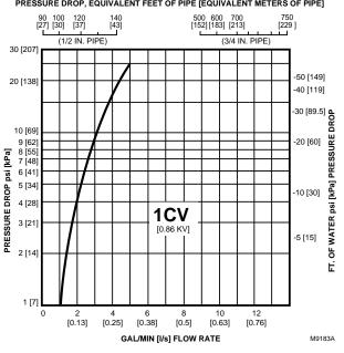
Fig. 55—Flow characteristics of 1 Cv [0.86 kV] valve.
