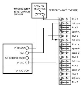
T675 WIRING FOR CONVENTIONAL FORCED AIR SYSTEMS M8169
