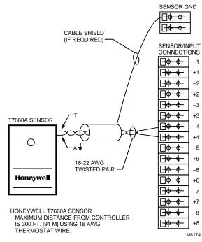
Fig. 42—Typical T7660B Space Temperature Sensor wiring.
