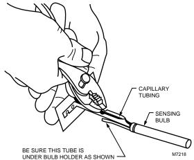
Fig. 33—Securing the bulb to the bulb holder.
