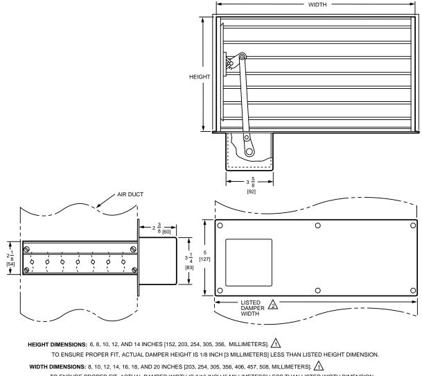
Fig. 12—Automatic opposed blade damper-bottom mount dimensions.
