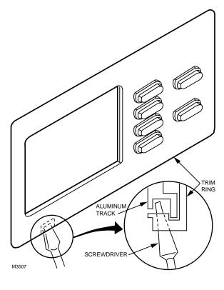
3. Mount the Touchpad in a 3-gang junction box or drywall as follows:
