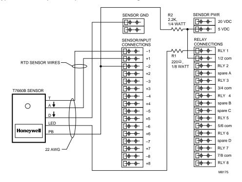
Fig. 41—Typical T7660A Space Temperature Sensor wiring.
