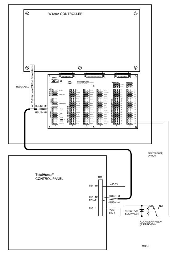
Fig. 29. Wiring between TotalHome<sup>®</sup> and W180A Controller.
