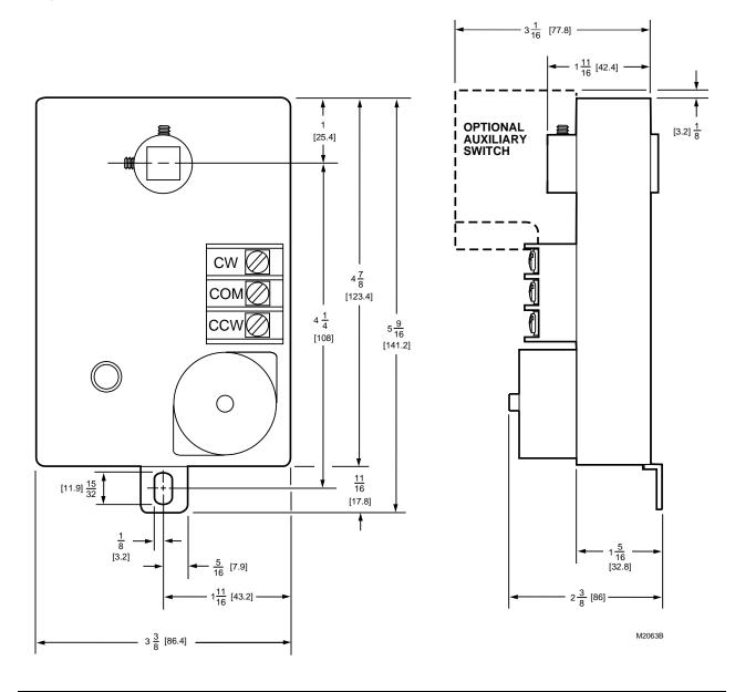
Fig. 10—ML6161 Direct Coupled Actuator dimensions in in. [mm].
