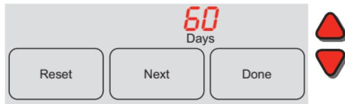
If activated during installation, the furnace filter reminder alerts you when it is time to replace your filter.
