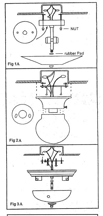
NOTE: The above diagram illustrates the installation of your new lighting fixture. This is a representative drawing and is not intended to match the style of your fixture.
