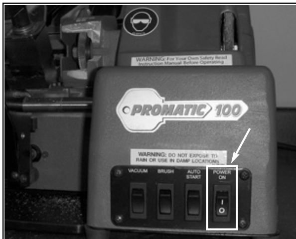
Turn the main power back on while...
