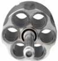
Carbon rings left behind by ordinary gun cleaner.
