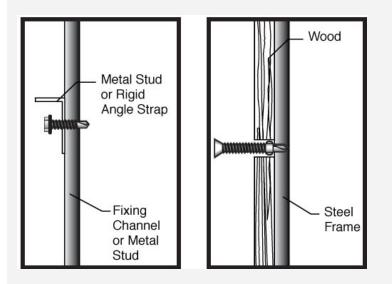
**Self Piercing Screws -** designed for use in thin sections of metal, 20 gauge or less. The point "punctures" through the material, allowing the threads to protrude through the metal, reducing the possibility of "strip-out." Self Piercing Screws are available in the following forms: Hex Washer Head, Framing and Lath Screws, Self Piercing Sheeters (Polebarn) and Stovepipe/Gutter Assembly Screws.
