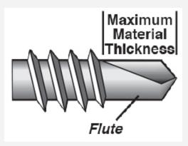
**Self Drilling Screws -** designed for power driving wood or metal to metal without drilling a pilot hole. The Drill Point drills it's own hole, taps mating threads and fastens firmly in one operation. Drill Screws penetrate 18 gauge steel or greater. Drill screws are available in the following styles: Pan Head, Hex Washer Head, Flat Head, Wafer Head, Framing and Lath Screws.
