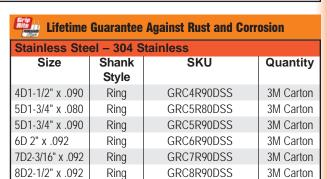
Only stainless steel fasteners are recommended for use with cedar and redwood, and carry a lifetim guarantee against rust and corrosion when used with these materials.
