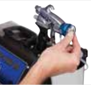
1) Remove front air cap and nozzle
