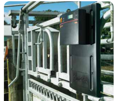
Integrated BR Series and Weigh Scale Indicator system on cattle handler.
