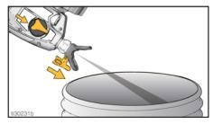
Reverse the Spray Tip to UNCLOG position, pull the Trigger for 30 seconds until sprayer is clean. Release the Trigger.
