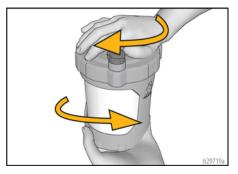
4. Verify Pump Filter is installed and clean.
