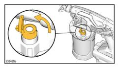
e. Tilt sprayer so the VacuValve is the highest point.
