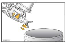
Turn Prime Knob forward to SPRAY position. Rotate Spray Tip 180 degrees to UNCLOG position.
