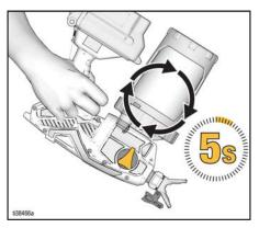
d. Turn sprayer upright and open the VacuValve Cap.
