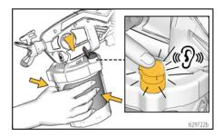
**NOTE:** If FlexLiner is not squeezed while VacuValve Cap is open, air will quickly pull into the FlexLiner. If any air bubbles are visible in the cup, repeat steps E-G. 7. Turn Prime Knob forward to SPRAY position. Verify Spray Tip is forward in the SPRAY position.
