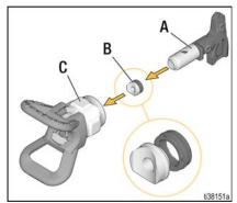
Insert Spray Tip into Spray Tip Guard. Verify Spray Tip is forward in the SPRAY position.
