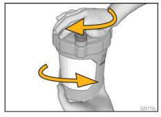
8. Install the cup onto the sprayer.
