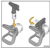
4. Screw Spray Tip Guard assembly onto sprayer and hand tighten.
