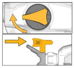
While holding the sprayer upside down, point the sprayer into a waste bucket. Pull the Trigger for 30 seconds.
