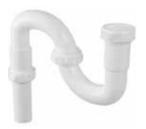
Used in kitchen sink and washbasin applications where plumbing connection is made at floor. Adaptable  $1\frac{1}{2}$ " x  $1\frac{1}{4}$ " washer included in P/N 177151. Can be utilized to connect  $1\frac{1}{2}$ " tubes,  $1\frac{1}{4}$ " tubes, as well as adapt from  $1\frac{1}{2}$ " to  $1\frac{1}{4}$ " tubes.
