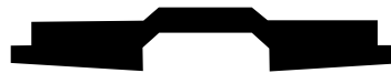
TYPE 29 Flap disc with a flexible design for smoothing and grinding contoured surfaces
