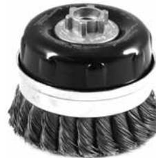
Ideal for heavy-duty cleaning of metal surfaces. Made from high carbon tempered steel. Equipped with metal bridle to eliminate flaring. When wire is worn to the metal bridle, it can be knocked off by a hammer blow exposing more wire for 30% longer life.
