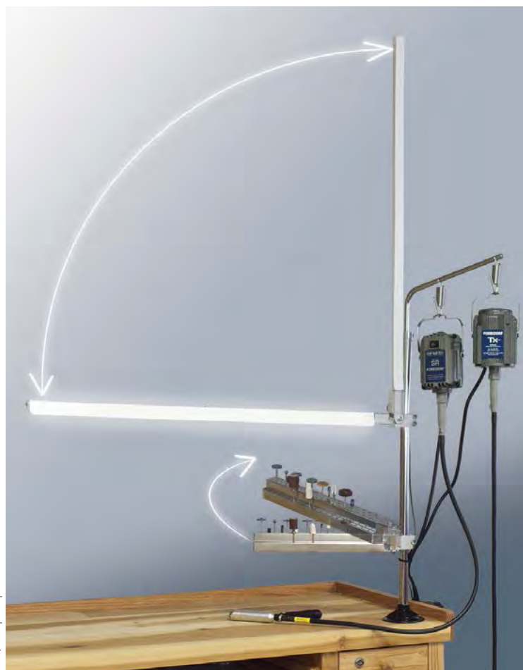
When MALB-1 Light Bar is horizontal it is ON – pivoted 90° upright, it turns OFF .
